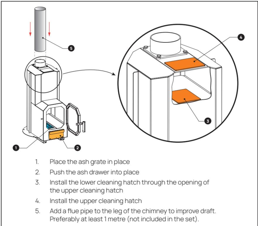
**Figure 5.** Assembling the stove for pre-installation heating.
