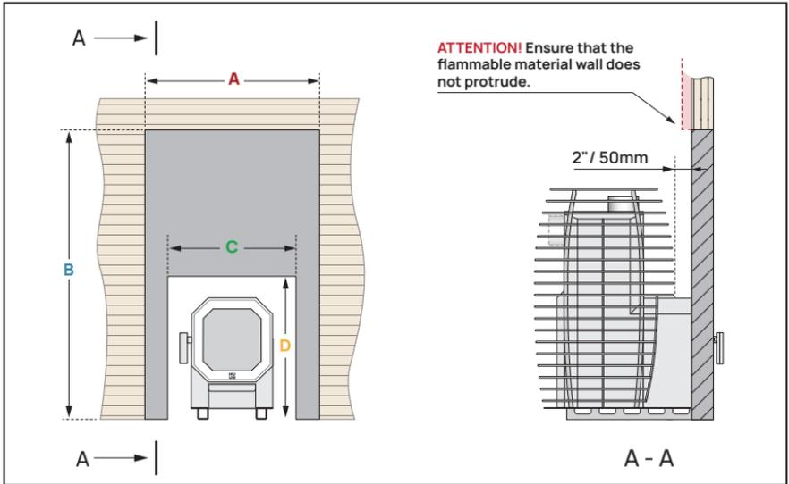
Figure 9. Installing HIVE Flow LS and Flow Mini LS sauna stoves through the wall.
