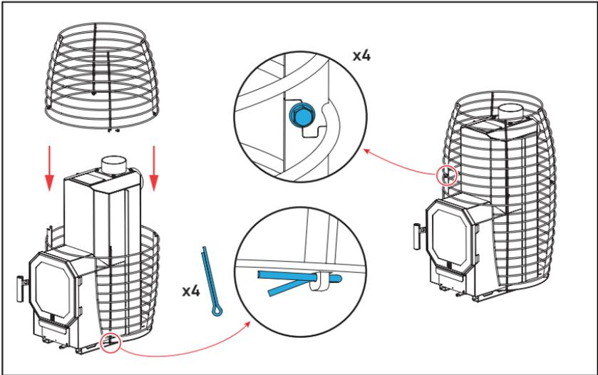
Figure 13. Splitting HIVE Flow stone grid.
