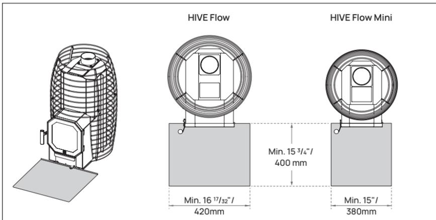
**Figure 8.** HIVE Flow and Flow Mini sheet metal plate for floor protection (sold separately).
