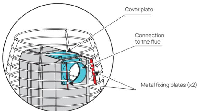
**Figure 10.** HIVE Flow back connection. The two ribs should be cut according to the diameter of the chimney element and the loose ends of the ribs should be fixed with the metal fixing plates found in the package.
