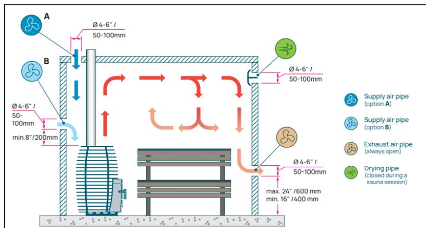
Figure 12. Mechanical ventilation in a wood-fired sauna
