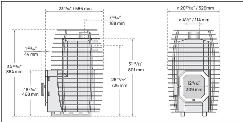
**Figure 1.** Dimensions of the HIVE Flow sauna stove.
