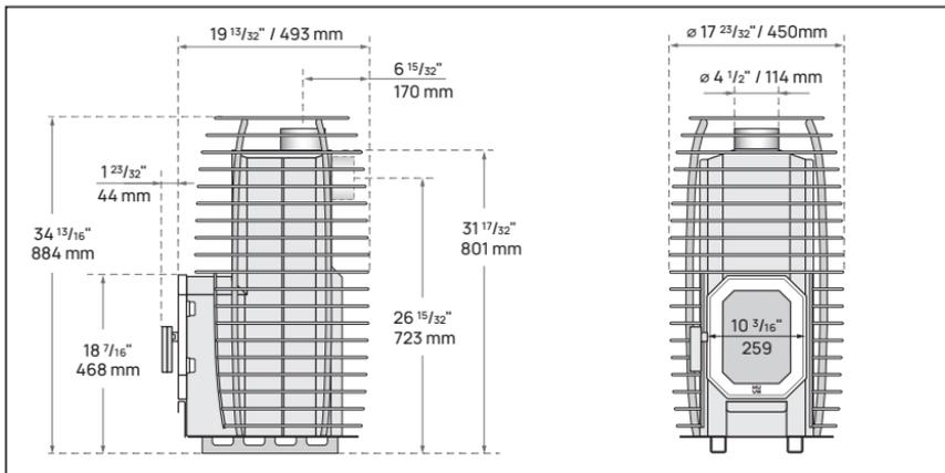
**Figure 3.** Dimensions of the HIVE Flow Mini sauna stove.
