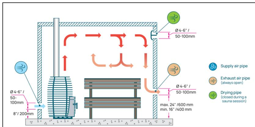
Figure 11. Gravity-based ventilation in a wood-fired sauna
