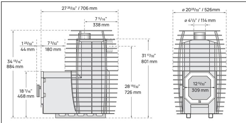
**Figure 2.** Dimensions of the HIVE Flow LS sauna stove.
