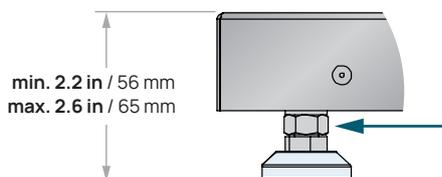
**ENG** The nut must be screwed against the bottom of the plate.
